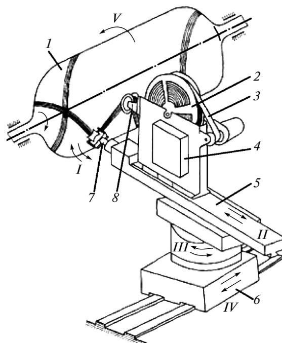
**Fig. 3.** Scheme of "dry" winding of article: (1) mounting, (2) bobbin with prepreg, (3) dividing film, (4) heater, (5) support, (6) carriage, (7) head, and (8) tension device.
