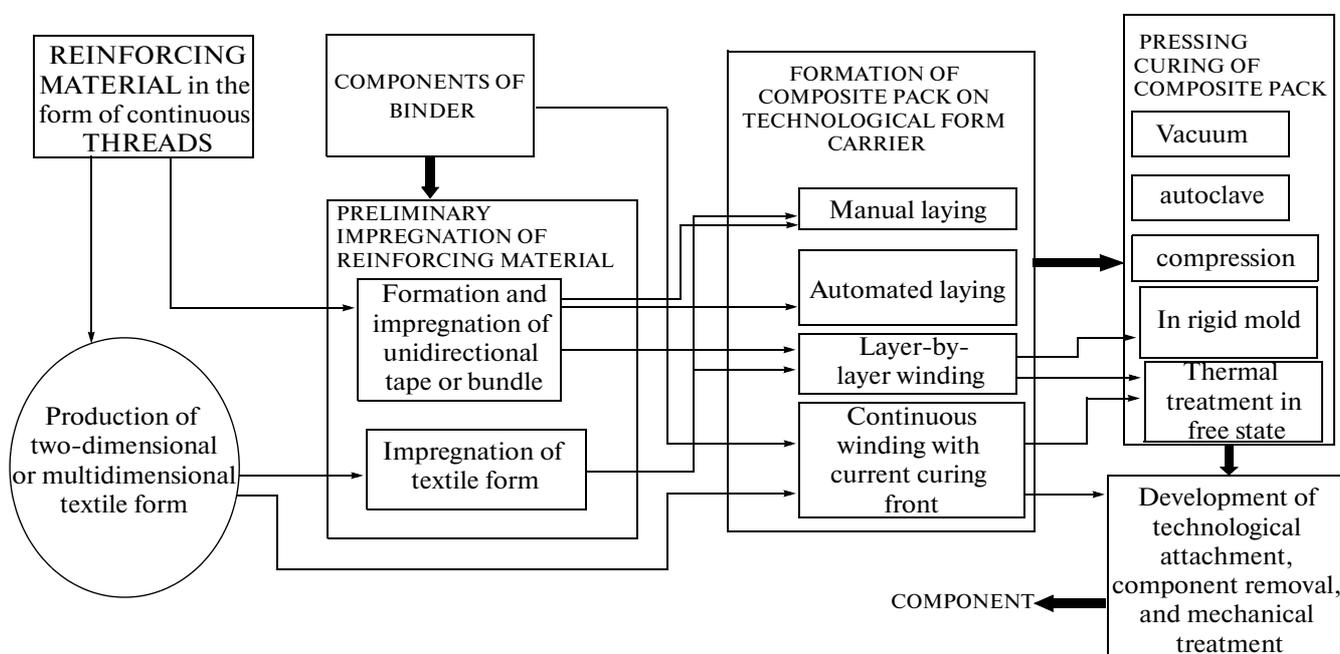
Fig. 1. Principle scheme of process of component production from PCM with the use of prepregs.
