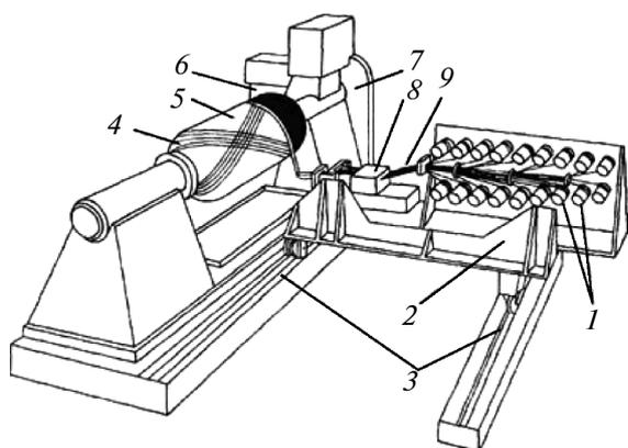
**Fig. 2.** Scheme of "wet" winding of component: (1) bobbin with threads, (2) bobbin holder, (3) laying-impregnating section, (4) helical layers, (5) mount, (6) circumferential layers, (7) rotary drive, (8) bath with binder, and (9) formed unidirectional tape.
