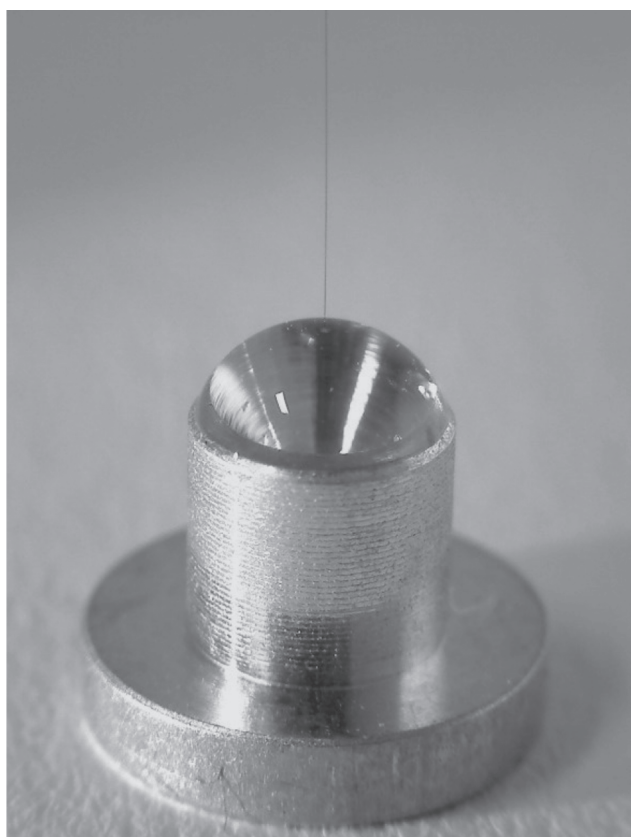
Fig. 2. Photo of a device for preparation of samples with cured epoxy binder for their subsequent pull-out tests. An elementary filament is fixed inside it.
